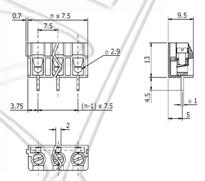
Recommended PCB holes diameter: f 1.2 mm to f 1.4 mm
