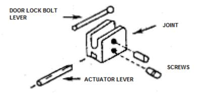
Figure 3. Connecting levers with joint
