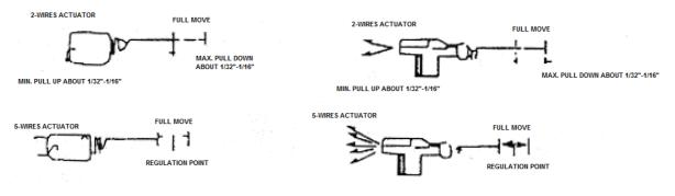
Figure 4. Actuator stroke regulation
