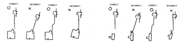
Figure 2. Actuator and door lock levers position
