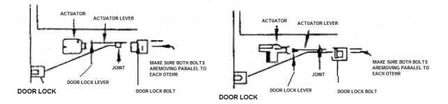
Figure 1-b. Actuator installation example
