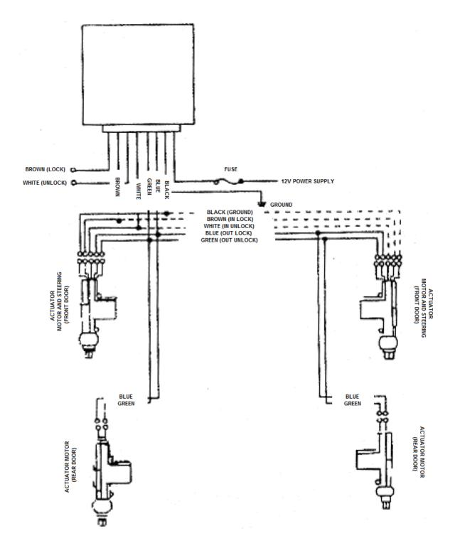
Figure 5. Wires connection
