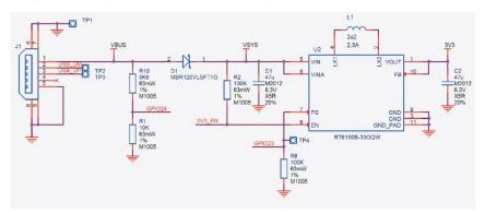
VBUS is the 5V input from the micro-USB port, which is fed through a Schottky diode to generate VSYS. The VBUS to VSYS diode (D1) adds flexibility by allowing power ORing of different supplies into VSYS.
