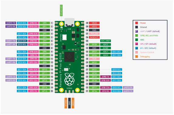
Pico uses an on-board buck-boost SMPS which is able to generate the required 3.3V (to power RP2040 and external circuitry) from a wide range of input voltages (~1.8 to 5.5V). This allows significant flexibility in powering the unit from various sources such as a single Lithium-Ion cell, or 3 AA cells in series. Battery chargers can also be very easily integrated with the Pico powerchain.
